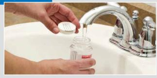
TURN THE WATER DOWN so it does not splash. Fill the bottle to the fill line (100 ml). Keep the bottle under the stream of water; DO NOT touch the bottle to the faucet. Do not fill it all the way up to the top.
